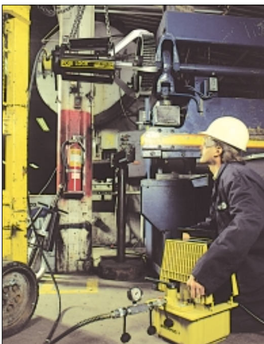
◀ An EPHR-116, 50 ton hydraulic Posi Lock® puller easily removes the main drive gear from this metal forming brake press.
